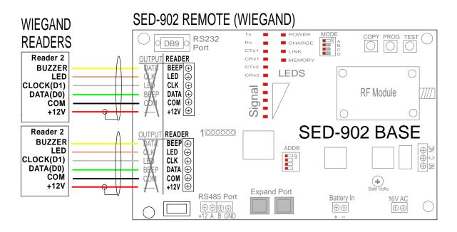
**IMPORTANT**: If using the SED-902 system on a Gallagher controller with a Wiegand reader adaptor, or a Wiegand system which does not use the standard logic levels of 0-5V, then  $2.2k\Omega$  pull up resistors must be fitted on the Master/Expander between the Clock and 12V terminals, as well as Data and 12V terminals.
