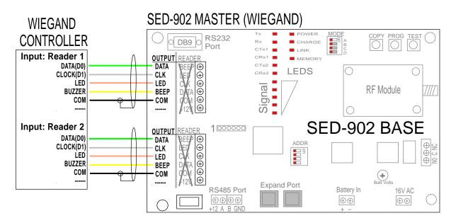
**IMPORTANT**: If using the SED-902 system on a Gallagher controller with a Wiegand reader adaptor, or a Wiegand system which does not use the standard logic levels of 0-5V, then  $2.2k\Omega$  pull up resistors must be fitted on the Master/Expander between the Clock and 12V terminals, as well as Data and 12V terminals.
